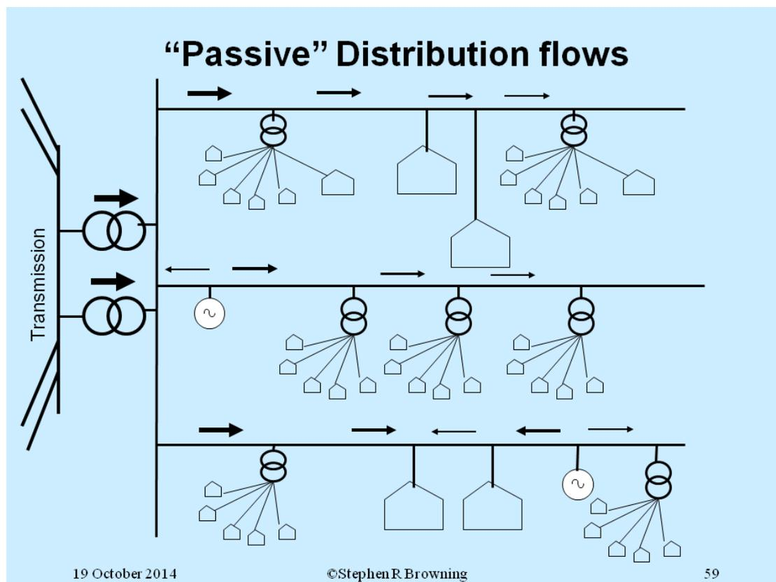
GB domestic feeders at 240V are 60A/phase 14kW and 100A/phase 25kW.
